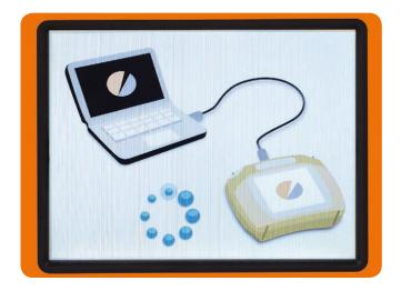
Noises which have been recorded can be played back using the player integrated into **WaterCom**. If the software is used regularly to save measurements, it will start to build up a useful noise database. This can then be used, for example, to train new starters in leak detection in what to listen out for.
