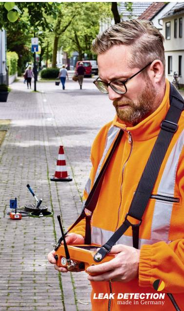
The **SeCorrPhon AC 200** is a multifunctional leak detector offering three functions in one: prelocation, pinpointing and correlation. The clever combination of these processes in one system allows you to confidently locate the leak regardless of the ambient conditions. With just a few finger strokes, you can quickly and easily switch between the various applications.
