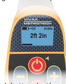
Push button depth reading
