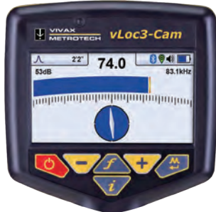
Pushrod Trace mode - Locate the pushrod or buried utilities
