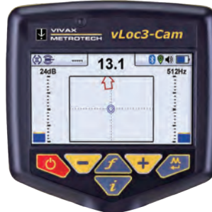
Directional arrows point to the sonde location
