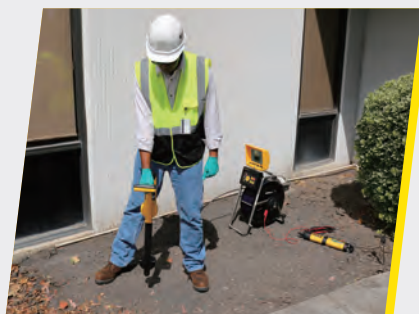
Locatable pushrod and sonde
