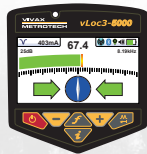
A green bar graph indicates clean locating conditions with very low distortion
