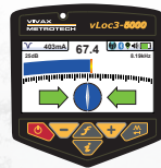
A blue bar graph indicates a medium level of distortion
