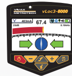
A red bar graph indicates very high distortion. Both Peak and Null locates are subject to significant positional errors
