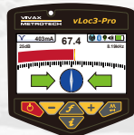
A red bar graph indicates very high distortion. Both Peak and Null locates are subject to significant positional errors
