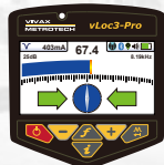
A blue bar graph indicates a medium level of distortion
