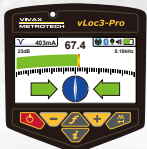
A green bar graph indicates clean locating conditions with very low distortion
