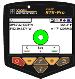
Aligned GNSS Antenna
