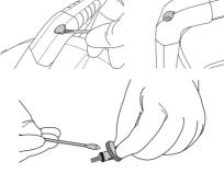
3. Align the adapter's alignment pin with the slot in the handle and press the adapter in place.
